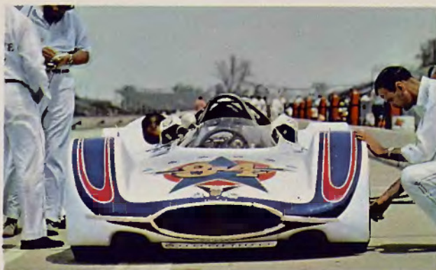
Mickey Thompson's Ford-powered Indy car had enclosed wheels.
