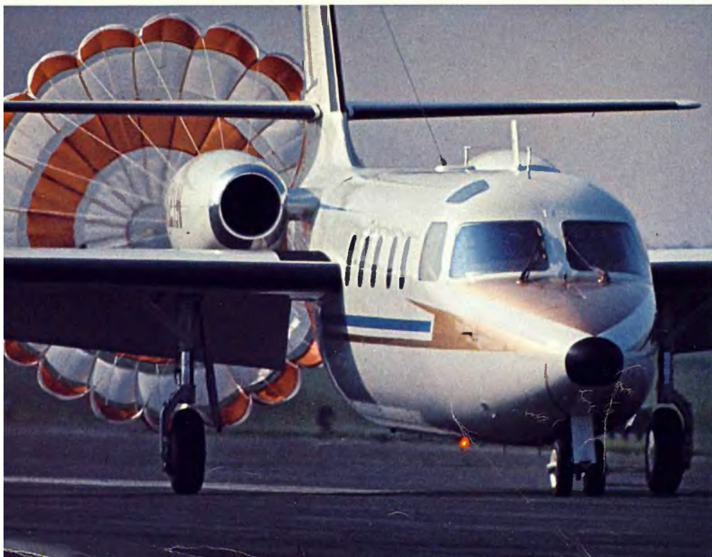
COMMODORE: Israel Aircraft Industries builds this plane, shown at left landing with deceleration-aiding parachute billowing behind. The Commodore has been improved recently with the introduction of model 1123, a larger and more powerful business jet than its predecessor, the 1121.
