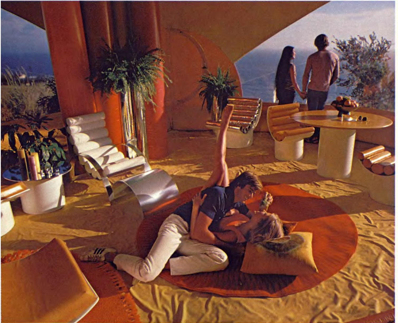
118 Above: A panoramic vista of the Pacific complements the dramatic interior of the Pseudome; a blower hooked up to the house keeps it inflated and dust-free. The multicolored vertical fiberboard cylinders at the rear of the room are not structural but act as space dividers.
