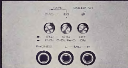
Separate bias and equalization switches for any type of tape.
