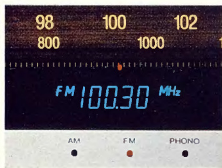
Sony's exclusive fluorescent Digital Plus display moves with dial pointer.
