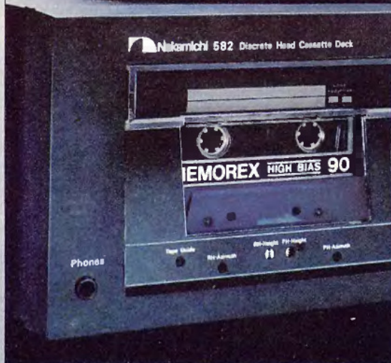
The GenRad 1995 Integrating Real-Time Analyzer measured signals from a Nakamichi 582 cassette deck. Input signal source was "pink noise" at OdB (200 nanowebers—standard record level).
