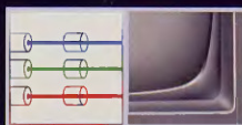
Conventional three-lens system. Focus is limited by the small size of its lens—its spherical screen distorts the shape of the picture, while cutting the image off at the corners.
