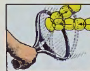
Aluminum and fiberglass largehead frames flex more, sending the ball in off-target directions.
