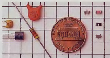
In PASSPORT, 102 SMDs (right) do the work of ordinary transistors, resistors and capacitors.
