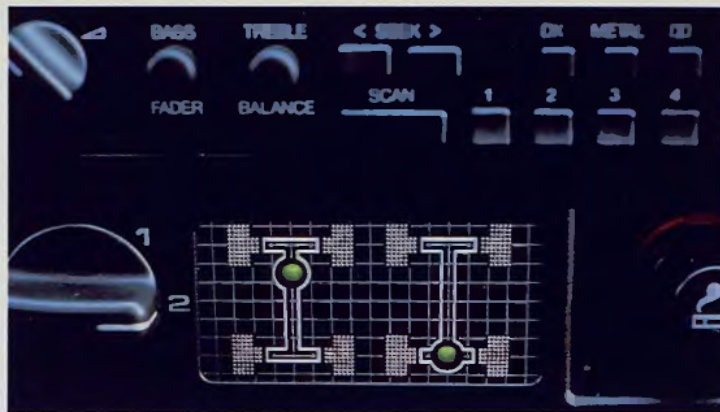
A view of the Audi 5000CS Turbo Quattro's console-mounted differential lockup. With a fully locked-up differential, both wheels on the same axle are locked in the same orbit. If one is slipping on ice, the other one turns as well, pulling you out of whatever you've gotten yourself into. Right: Six of the sportiest all-wheel-drive machines for you to dream of and drool over.
