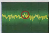
How a conventional superheterodyne radar detector sees a police radar signal.
