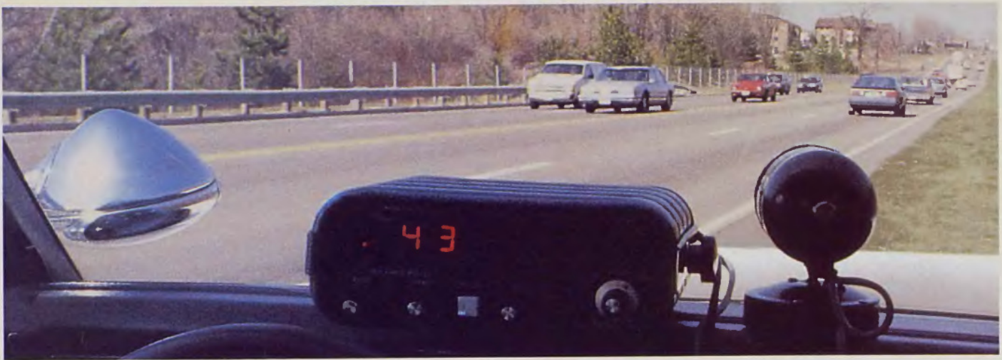
Traffic radar doesn't say which car is being clocked, it merely flashes a number. The radar operator must then try to determine which vehicle produced the reading.
