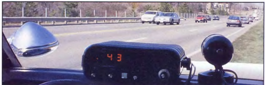
Since radar displays only one number, the operator has the responsibility to decide which vehicle is being clocked.
