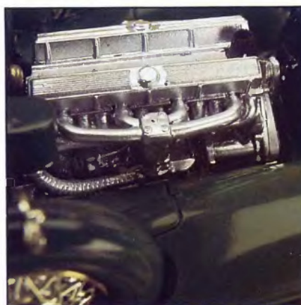
ENGINE: The detail of this 452 cubic inch, sixteen-cylinder overhead cam engine is authentic.
