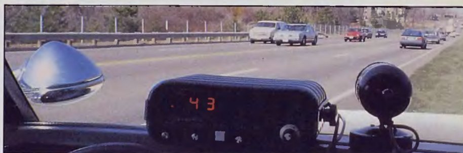
Since radar displays only one number, the operator has the responsibility to decide which vehicle is being clocked.
