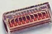
Instead of a conventional meter, SOLO uses ten Hewlett Packard AlGaAs LEDs bonded directly to a tiny circuit board.
