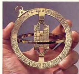
Finally, turn the entire dial until sunlight coming through the pinhole in the index is focused on the hour ring.
