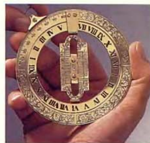
Begin by setting the suspension ring to the local latitude.
