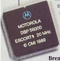
The heart of ESCORT's DSP circuitry is this 20 MHz 24 bit HCMOS processor, a custom version of the Motorola DSP 56000.
