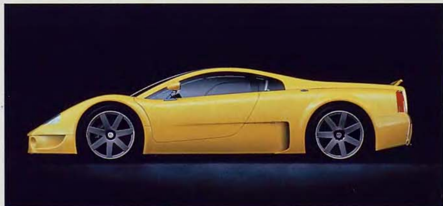
Below: Volkswagen and Italdesign's Fabrizio Guigiaro teamed up for this sports car shocker, the W12, from the "people's car" company. Its 48-valve, four-camshaft, 12-cylinder engine is a clever side-by-side alignment of two hopped-up VW VR6s netting 5.6 liters and 420 bhp. Power finds its way to all four wheels via a six-speed sequential manual gearbox. VW probably won't build this two-seater, but the compact engine will fit neatly in a future luxury sedan.
