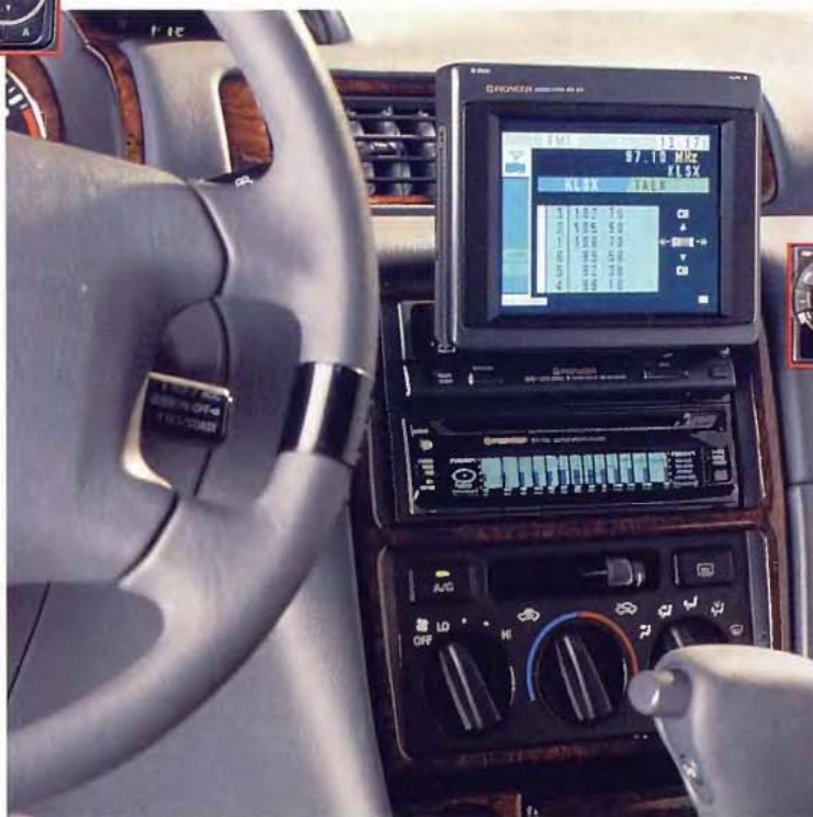
Pioneer's voice-controlled AVIC-505 navigation system keeps you on course with a global positioning satellite receiver, nationwide CD-ROM mapping software and a 5.6" color monitor that not only adjusts for the ideal viewing angle but also retracts when the system is not in use (about $2350).
