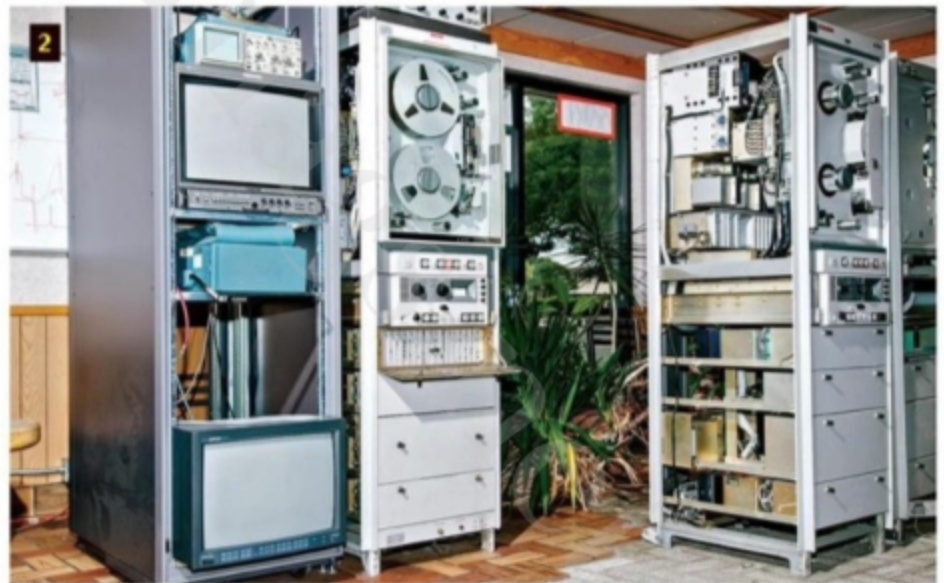
1. A decommissioned McDonald's serves as headquarters. 2. When scientists try to contact a space explorer launched 36 years ago, they need equipment equally old, like Ampex tape machines. 3. One scientist keeps his pet boxer, Major, on guard outside the tape vault and former freezer.
