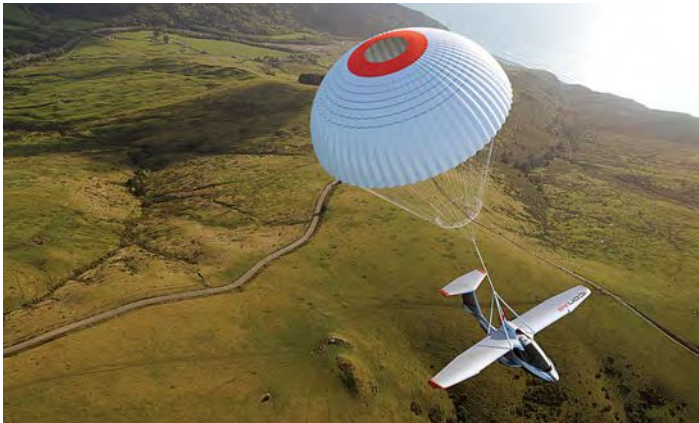
The Icon A5's controls resemble a Porsche's more than a plane's; the A5 has a safety parachute and is engineered for water and land takeoffs and landings.
